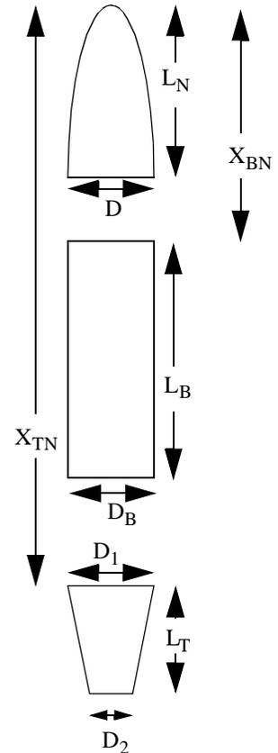
**Figure 1: Rocket Components**
